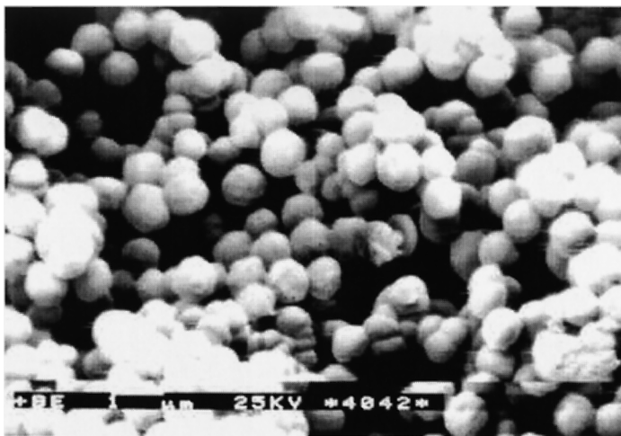
Fig. 2a.: SEM micrograph of PCHPMA microspheres prepared by dispersion polymerization in the presence of MPEG 5000 as stabilizer
